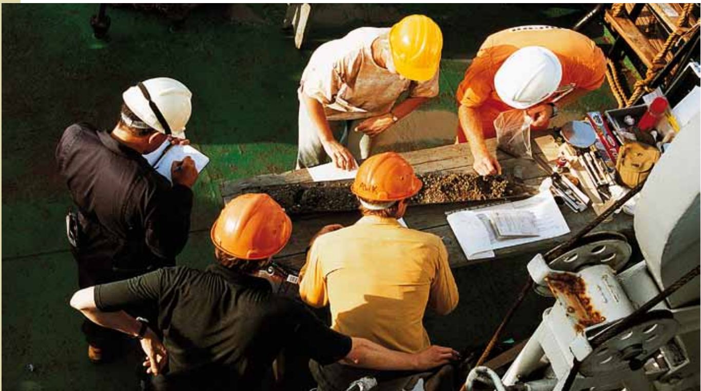
Figure 8 Core logging aboard the survey vessel (courtesy of Fugro Geoconsulting)
