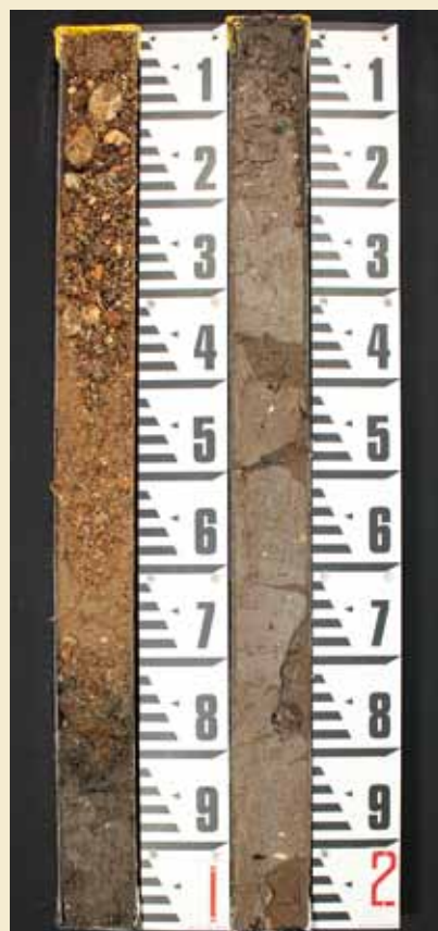
Figure 1 Split core samples showing sediment horizons (courtesy of Emu Ltd)
