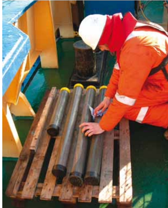
Figure 10 Labelling of vibrocore samples (courtesy of Emu Ltd)
