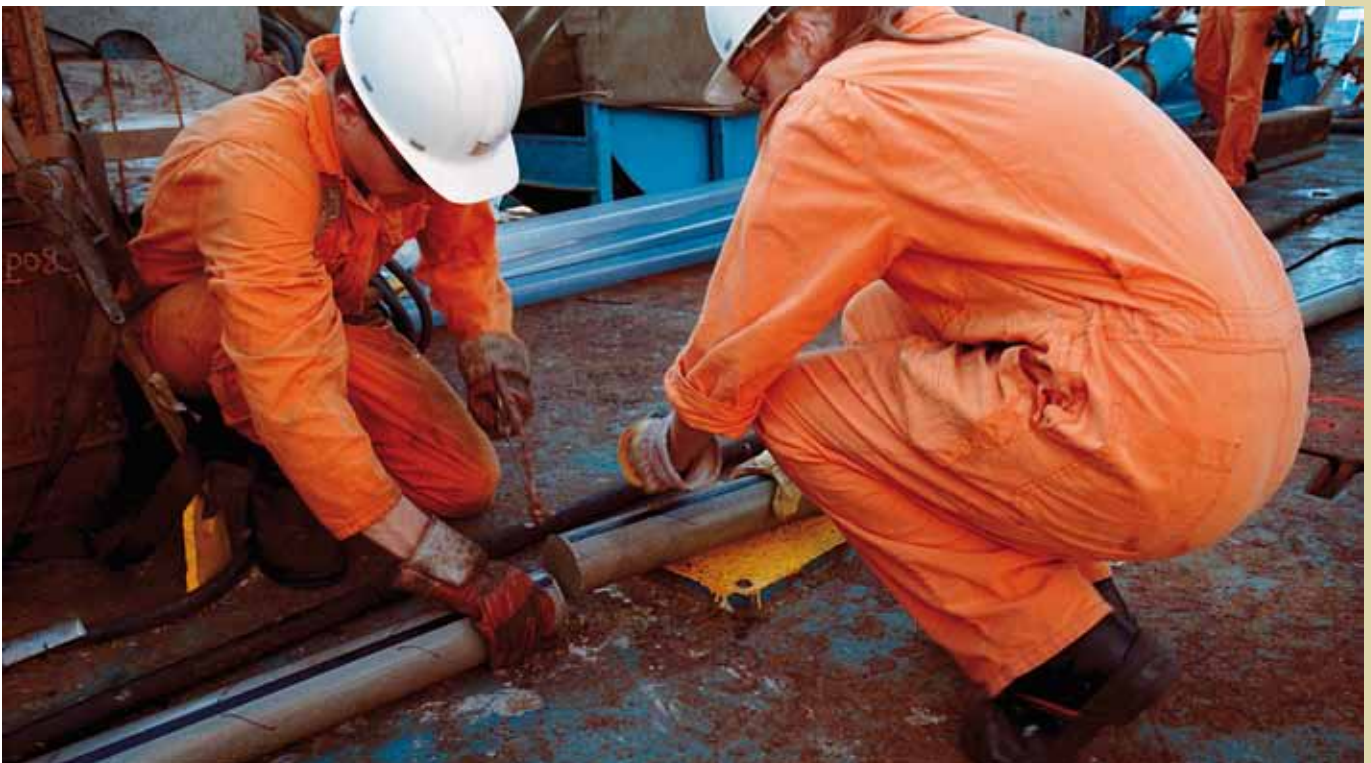
Figure 9 Vibrocore processing aboard survey vessel (courtesy of Fugro Geoconsulting)
