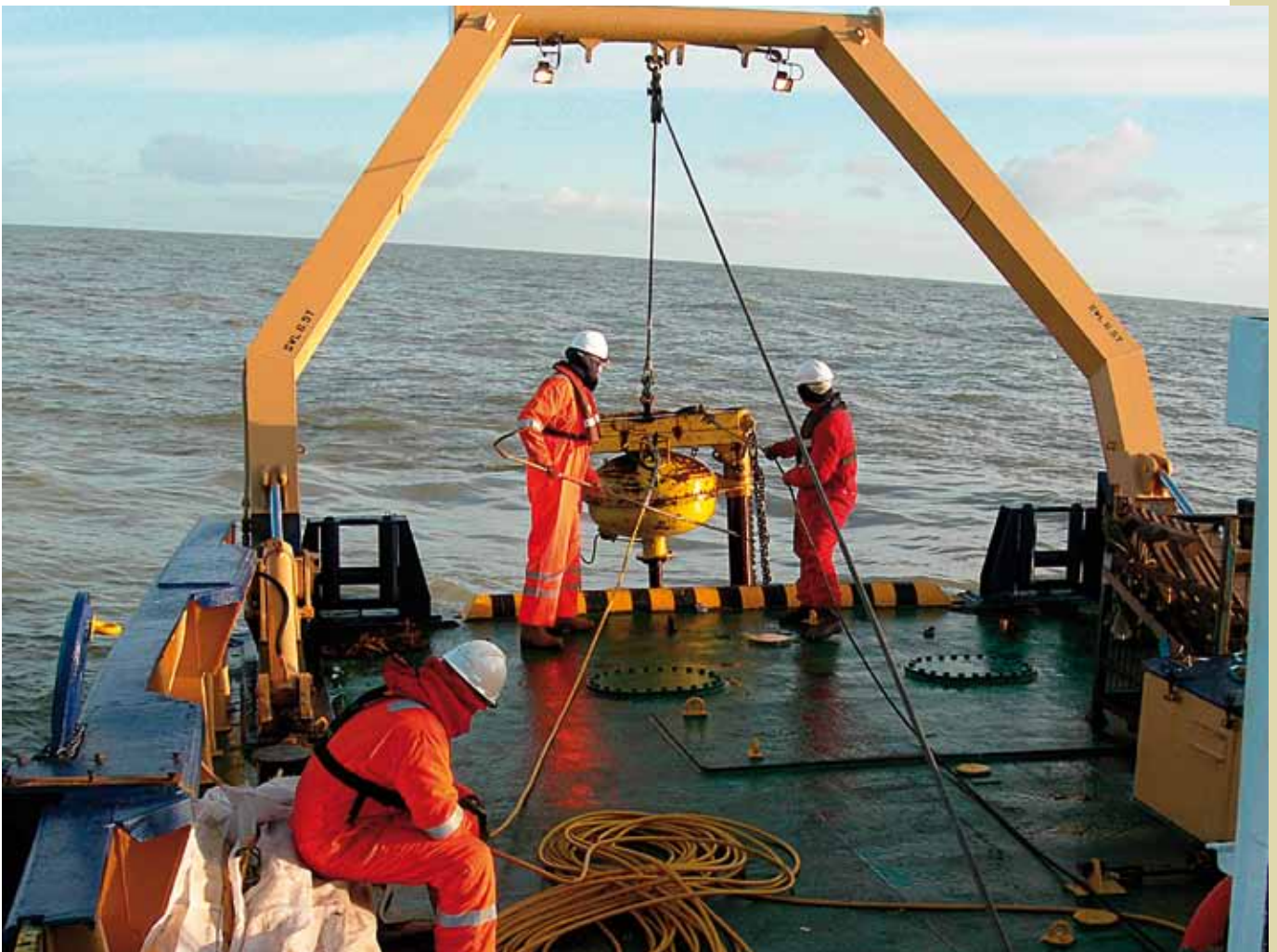
Figure 7b Vibrocorer deployment (courtesy of Emu Ltd)
