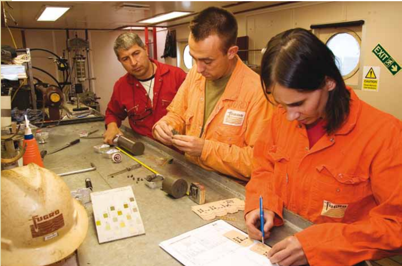
Figure 11 Offshore laboratory processing and testing of core samples (courtesy of Fugro Geoconsulting)
