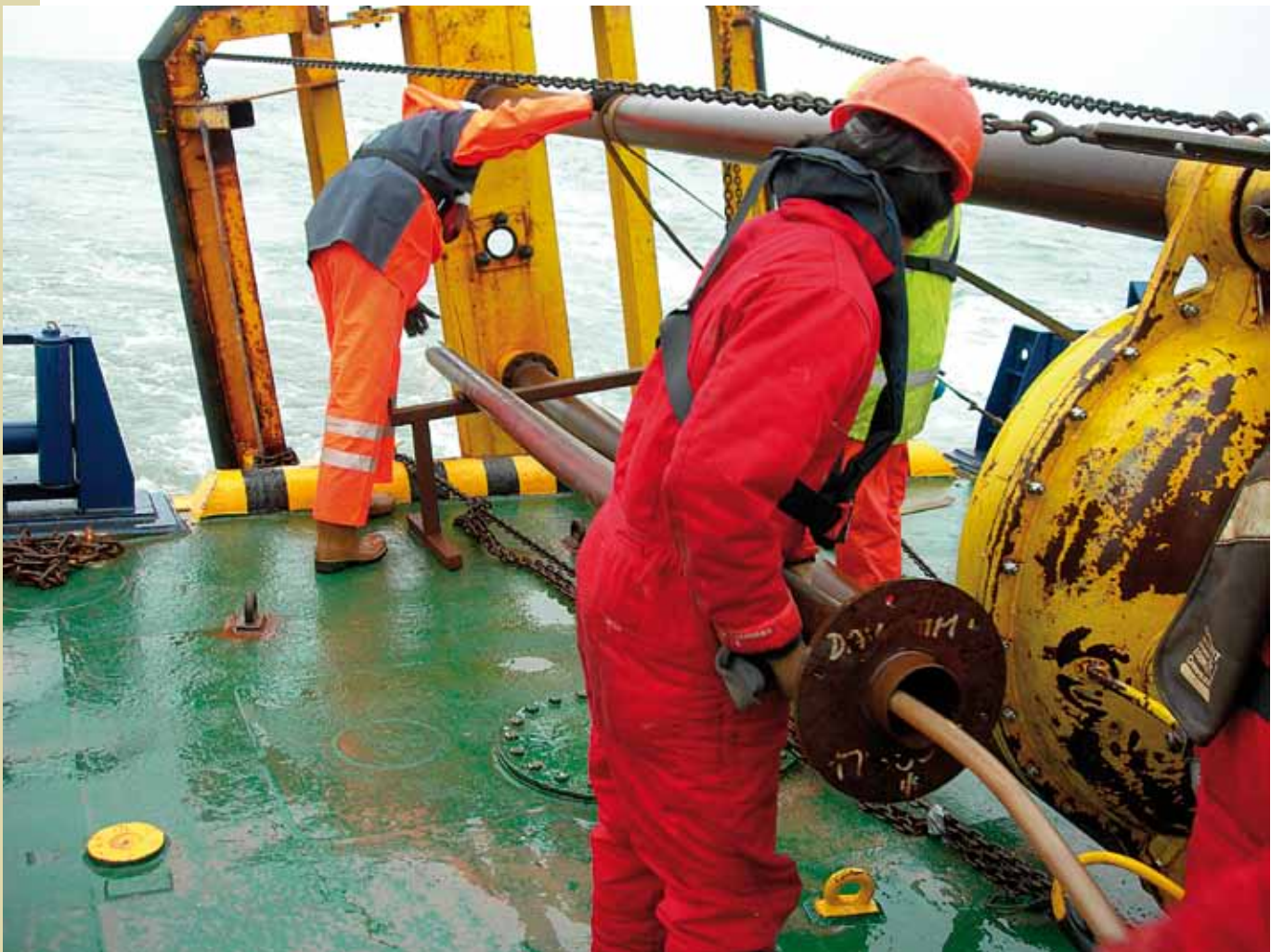
Figure 7a Vibrocorer set-up (courtesy of Emu Ltd)
